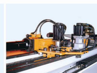
伺服強力輔推 (專利技術) Servo Controlled Strong POB Boost (Patented)
